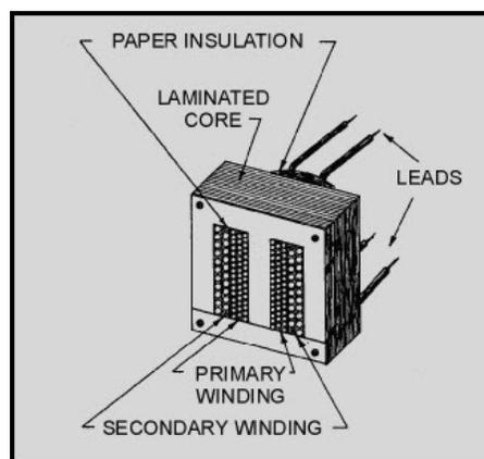
**Figure 5-6 Cutaway view of shell-type core with windings**
