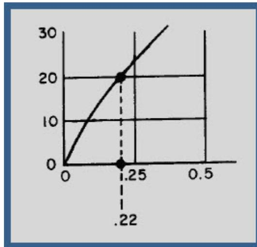
The value selected from the graph means that a capacitor (including the one you are solving for) will reach twenty percent of full charge in twenty-two one hundredths (.22) of one RC time constant. Remember that it takes  $100 \mu s$  for the capacitor to reach 20% of full charge. Since  $100 \mu s$  is equal to .22 RC (twenty two one-hundredths), then the time required to reach one RC time constant must be equal to:
