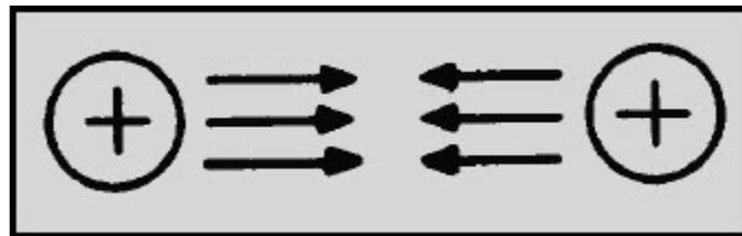
Figure 3-2 Electrostatic field repels two like charged particles
