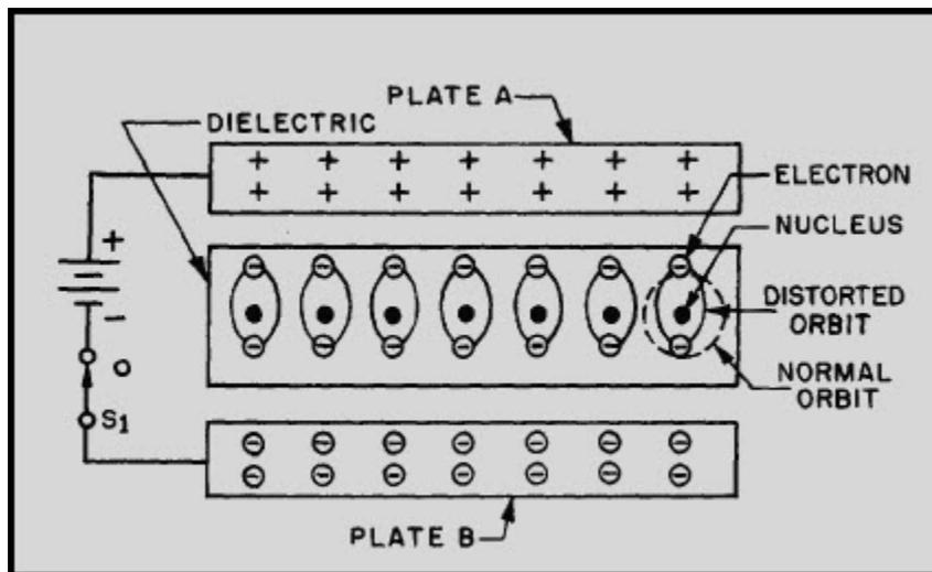
Figure 3-4 Distortion of electron orbits in a dielectric
