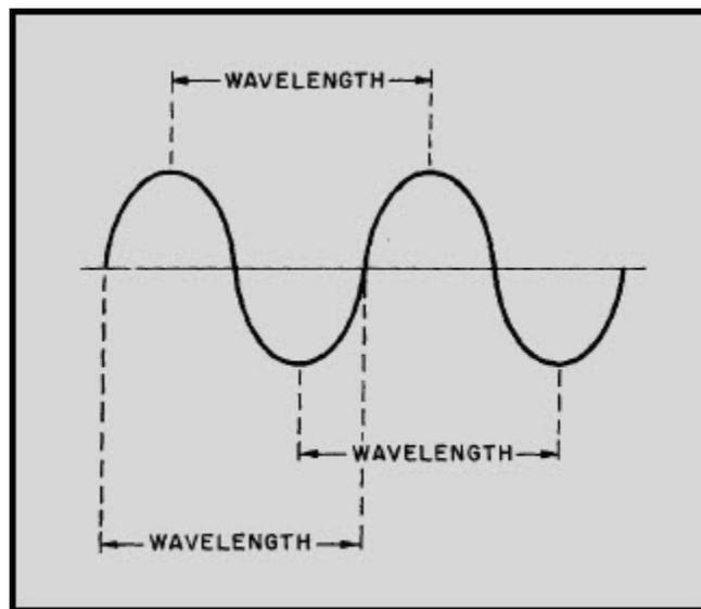
**Figure 1-12 Wavelength measurement**
