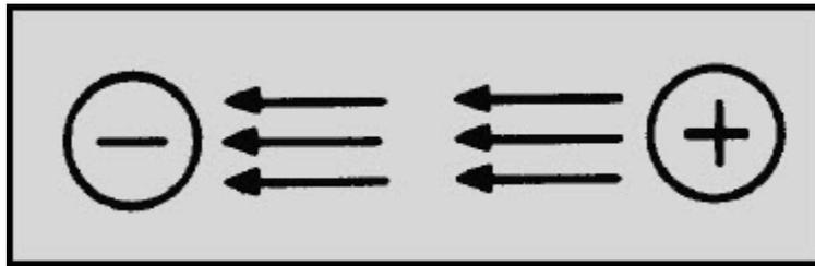
Figure 3-1 Electrostatic field attracts two unlike charged particles
