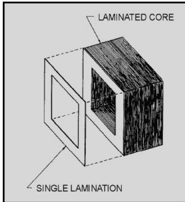
Figure 5-2 Hollow-core construction
