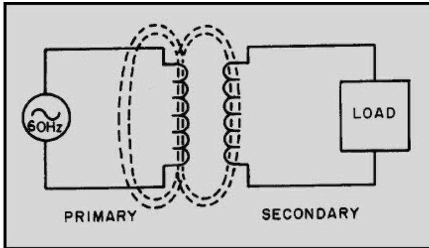
Figure 5-1 Basic transformer action
