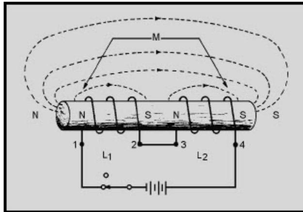
Figure 2-14 Series inductors with aiding fields
