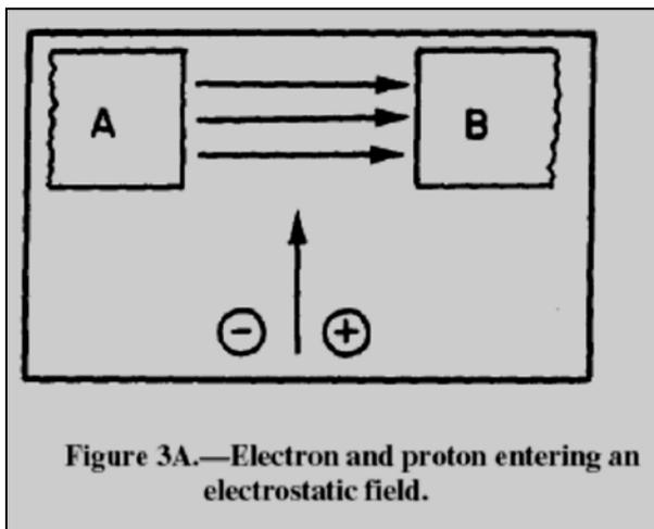
Figure 3A.—Electron and proton entering an electrostatic field.
