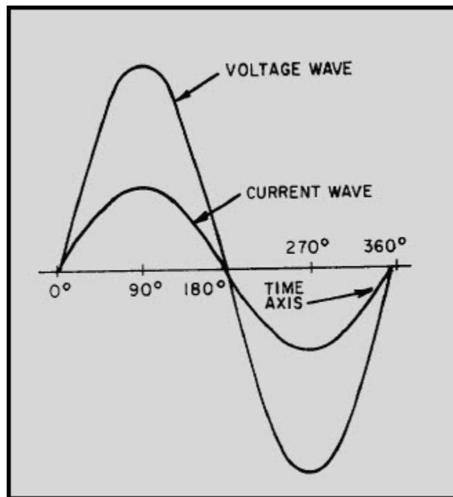
Figure 1-17 Voltage and current waves in phase
