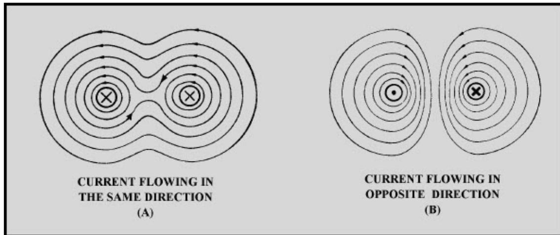
Figure 1-4 Magnetic field around two parallel conductors
