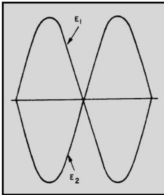
Figure 1-19 Voltage waves  $180^\circ$  out of phase
