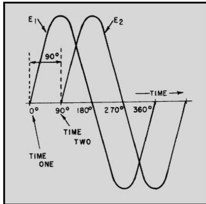
Figure 1-18 Voltage waves  $90^\circ$  out of phase
