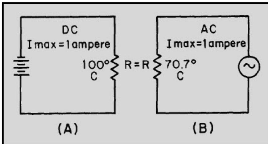
Figure 1-15 Heating effect of ac and dc
