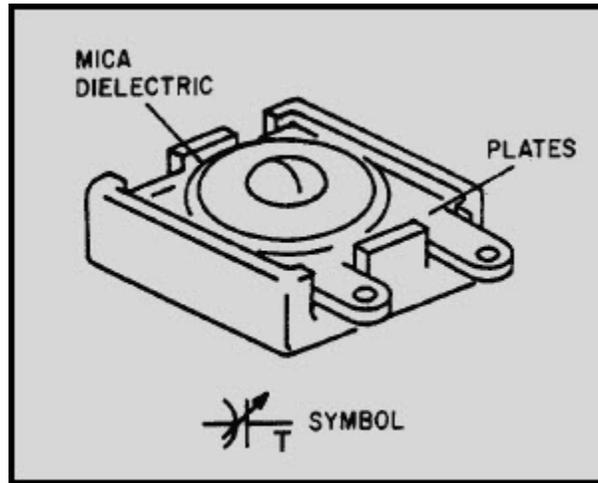
Figure 3-20 Trimmer capacitor
