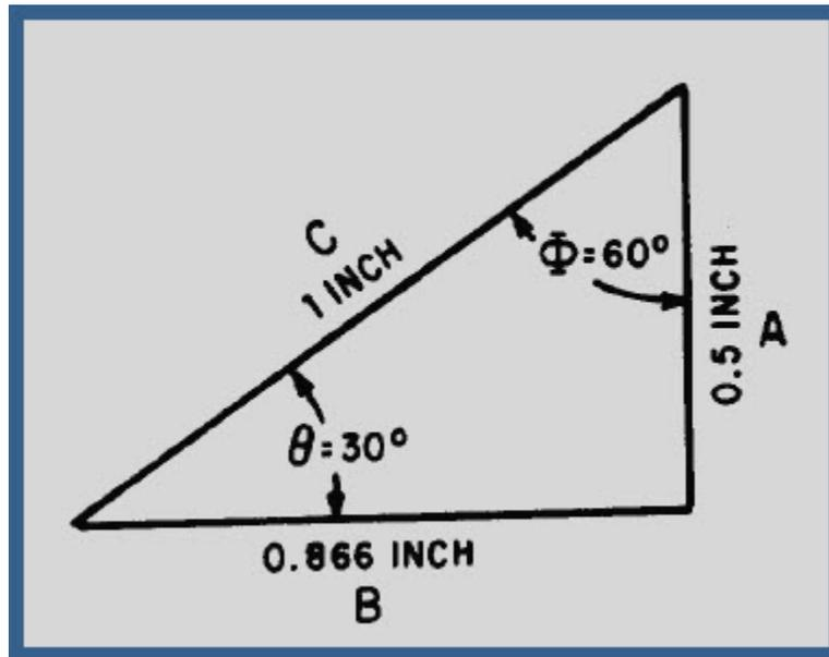
Figure 2 A  $30^\circ - 60^\circ - 90^\circ$  triangle
