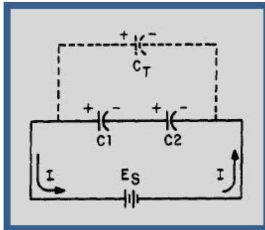
Figure 3-13 Capacitors in series
