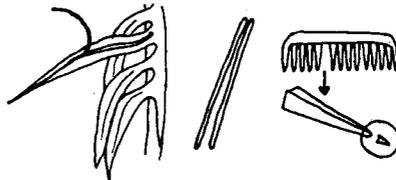
**5. Remove the extra cement before it gets too hard.** Press the flat side of the filling tool against the cement and smooth it towards the edge of the cavity.
