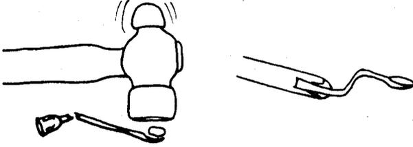
**Filling Tool:** Remove the heads from 2 long screws.
